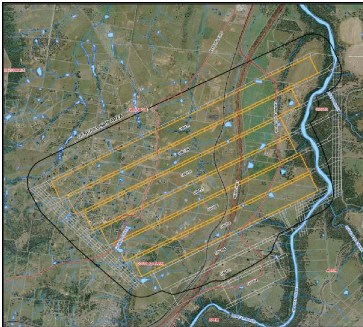
Figure 2.1 – Aerial Photograph Showing Longwalls 705 to 710 and the SMP Area
